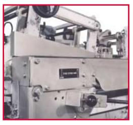
Two-position (straight or angle drop) panning section with manually locking device.
